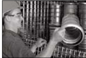
DROP GATE : A half-drop gate allows easy access and identification of parts.
