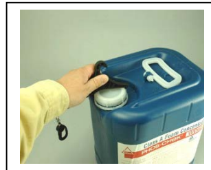
The above sequence of photos shows the 4577 Wrench being used to crack open a standard 5 gallon foam bucket.
