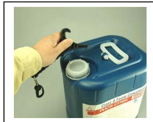
The above sequence of photos shows the 4577 Wrench being used to crack open a standard 5 gallon foam bucket.
