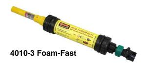
more efficiently. When connected to a 3/4" garden hose, the 4010-3 Foam-Fast™ works by diluting a solid foam cartridge in the water flow. The foam/water solution then passes through an air-aspirating foam nozzle producing foam suitable for Class A fires. Each Foam-Fast™ unit comes with six foam cartridges. Each 6" long foam cartridge will last up to one hour. The foam cartridges are 100% biodegradable and contain no toxic materials.
