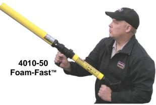
To operate, open the inlet side of the mixing chamber, insert a single 12" long foam cartridge, reseal the inlet end cap, attach to a hose, open the pistol grip shut-off and spray foam. The 4010 Foam-Fast™ is recommended for use with water pressures between 50 psi and 125 psi (maximum 150 psi).
