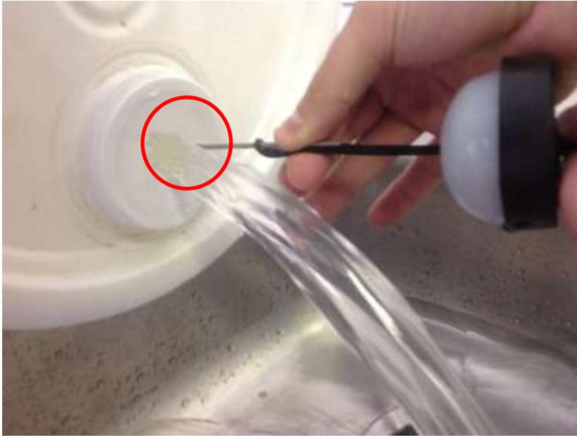
3. Slowly insert the pin into the rupture, quickly let go and remove the hand holding the pin so it is out of the path of escaping liquid.
