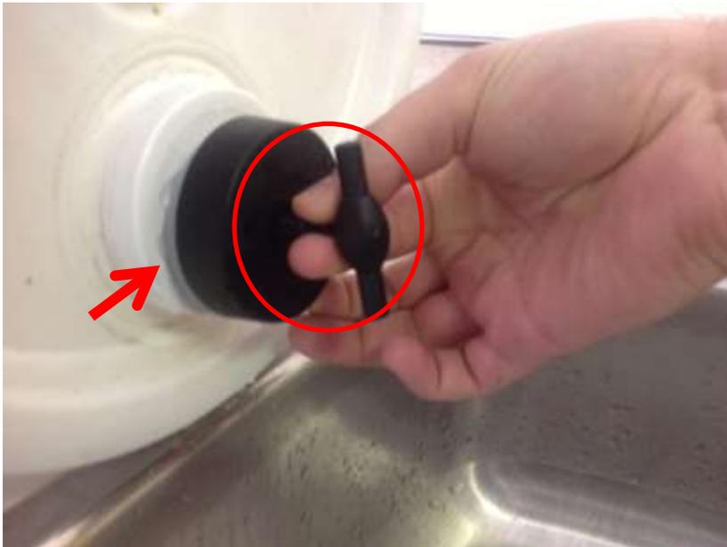
4. Force the RuptureSeal into the rupture and hold it in place creating a tight seal.
