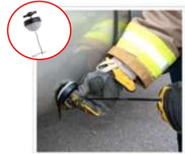
The RuptureSeal™ is an incredibly easy product to use, with one hand you flip the pin from the perpendicular position so that it is parallel to the tie, insert it into the rupture, and with the other hand hold the plug into the rupture, with your free hand pull on the handle until the clicking stops. The silicone is compressed into the rupture and takes the shape of the rupture whether it is smooth or uneven.
